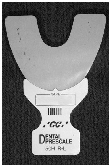
Figure 1— Pressure sensitive sheet (Dental Prescale).
